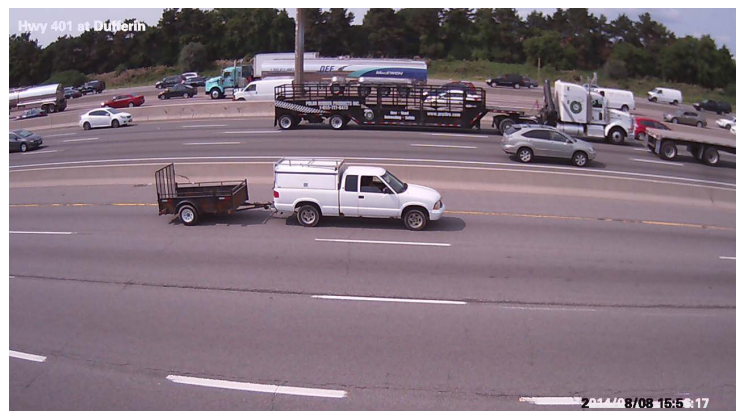
RTMS Sx-300 with IP camera provides visual verification during setup and data capture.
